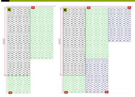
Lay further covers using the "laminate method" >> If an overlay is cut through, start the next strip with the remainder of the previous rubber cover. **Note** Make sure that you do not twist the rubber overlays when laying (see drawing, red markings).
