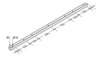
Drill holes with a diameter of 8 mm in the plastic moulding.
