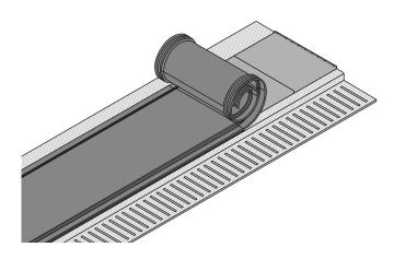
**Note:** If the cover sheet cannot be unrolled over the panels due to the installation, the unrolled sheet can also be pulled into position. Care must be taken to ensure that the foil is not damaged. The position of the composite foam plates should then be checked.
