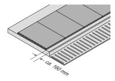
The foil-wrapped composite foam plates are laid at a distance of approx. 160 mm from the rear concrete edge.
