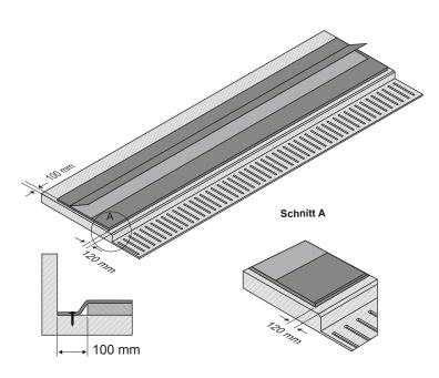
The composite foam panels are laid out with a distance of approx. 120 mm to the rear concrete edge. You need a distance of approx. 100 mm at the left and right ends. Then glue the foil to the composite foam panels.
