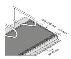
For fixing, holes are drilled in the cover sheet and the concrete. The distance to the edge of the cover sheet on the front side is 50 mm. The distance in the head and foot area is also 50 mm to the edge of the cover sheet. In between, further holes are drilled every approx. 200 mm and then the A2 8 x 80 nail plugs with washers are driven in.
