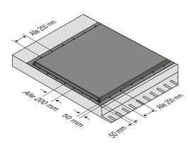
For fixing, holes are drilled in the cover sheet and the concrete. The distance to the edge of the cover sheet on the front side is 50 mm. The distance in the head and foot area is also 50 mm to the edge of the cover sheet. In between, further holes are drilled every approx. 200 mm and then the A2 8 x 80 nail plugs with washers are driven in.
