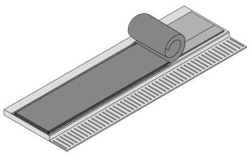
Unroll the composite foam panels and align them with a distance of 20 mm to the rear edge of the concrete.
