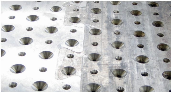
Sheet metal for comfort covering N20 (seam visible)
